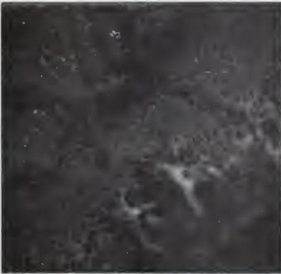
FIGURE 25. BIAxIAL COMPRESSIVE SPECIMEN FRACTURE SURFACE; EPON 828 + 10 pph CTBN R-151 (LARGE PAR- TICLES). (450X).
